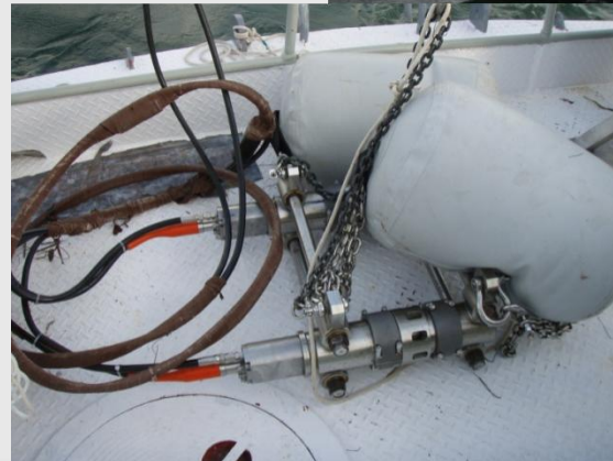
compressed air source, two 10 cu-inch Bolt airguns
